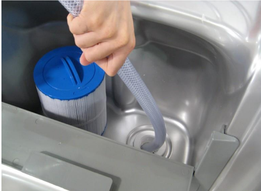
Figure 18. Filling Location in Filter Housing
